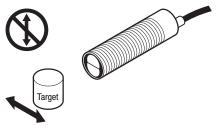
Note: Due to the detection method, targets traveling horizontal to the sensor's optics are detected. Targets traveling vertically may not be accurately detected. For reliable background suppression, a minimum separation distance of 6mm (0.24in) is recommended between the target and the backgrounds.
